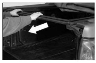
1. Remove the rear rail by pulling it straight out from the side rails. Set the rail aside.
